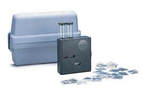
One of the least expensive, approved test kits is manufactured by Hach, and is the Model CN-66, Chlorine (Free & Total) Test Kit, with Color Disc, and reagents for 100 tests. Product #2231-01. Cost approximately \$44 not including shipping. Additional reagents can be ordered separately. Hach products are available from: Envirosource (A Division of Water & Ice Express), Guam; (671) 473-4374; fax (671) 473-4370; e-mail: johnlimtiaco@waterexpressguam.com or jenn\_limtiaco@waterexpressguam.com
